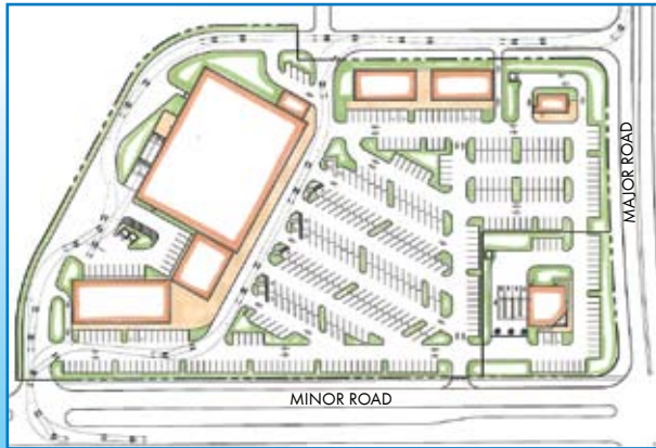
The first site plan was created using traditional design techniques with no regard for LEED criteria.
